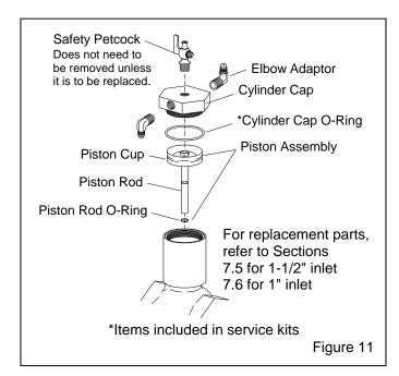
**5.1.2.6** Lubricate the cylinder wall and piston cup, with lightweight machine oil or tool oil.
