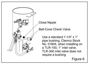
Note: Do not use a swing check valve, as the swing gate may break in blast machine applications. When installing the valve, make sure the directional arrow is pointing in the direction of the air flow (toward the machine).
