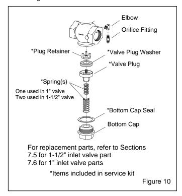
**5.1.1.4** Remove the lower twinline hose connection, and remove the orifice fitting for inspection. Clean the 1/16" orifice and reassemble the connection.
